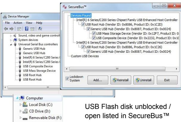
USB Flash disk unblocked / open listed in SecureBus™
